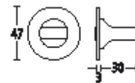
771/2531 Bathroom turn on concealed fixing rose for use with knob handles. Finishes: SS • PS • GT • BT • MA
